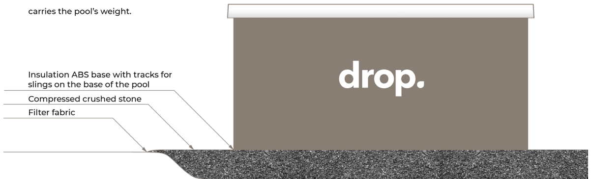
Please take into consideration the effect of frost when designing the base.
